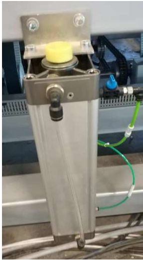
CUTTING OIL TANK
